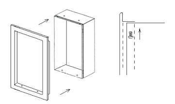
Prior to installing Door Trim, ensure that wall finishes are complete and that the door panel has been installed.
