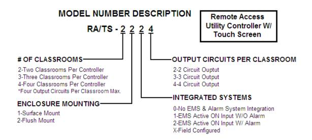
Note: All output circuits are low amperage. Interface relays are required for solenoid operation.
