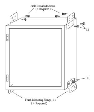
Figure 2 For best Flush Mounting results, recess face of enclosure's lip
